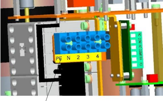
INTERNAL PROTECTION TERMINAL Fig 2b
