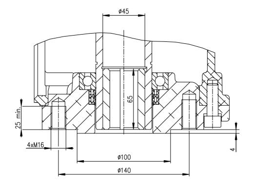
Connection dimensions **MO 4** with flange **«F14»** according to ISO 5210.
