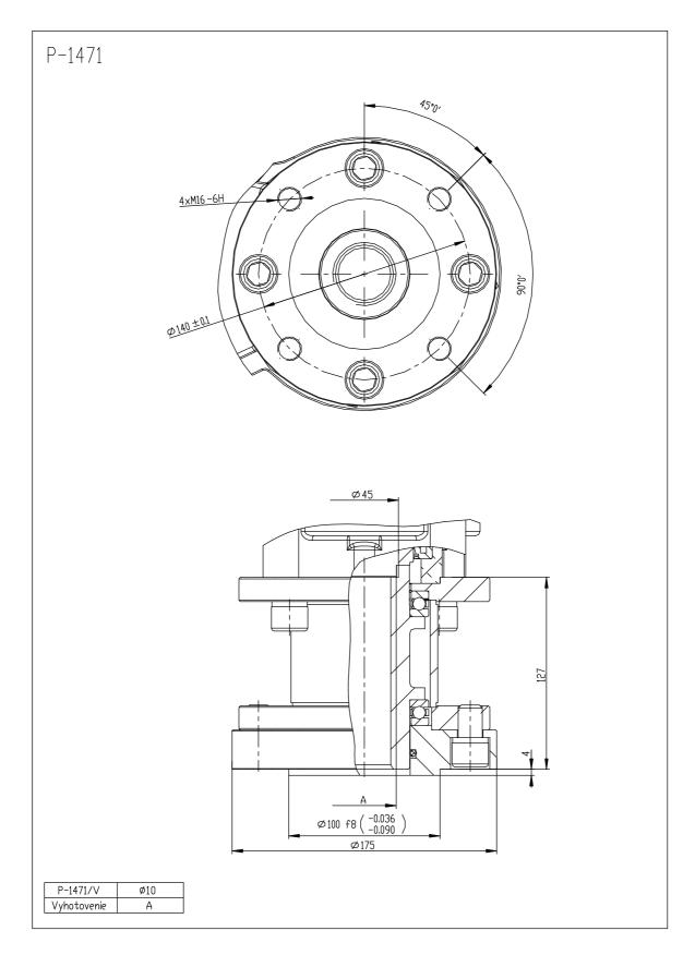
Connection dimensions MO 4 with flange **«F14»** according to ISO 5210. Shape of connecting detail **«B1»** ISO 5210.
