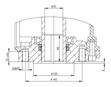
Connection dimensions MO 4 with flange «F14» according to ISO 5210.
