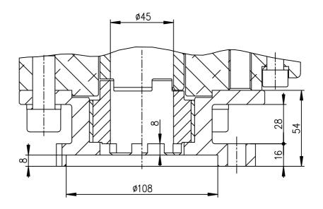
Connection dimensions **MO 4** with flange **«F14»** according to ISO 5210. Coupling shape **«B2 / B4»** ISO 5210.
