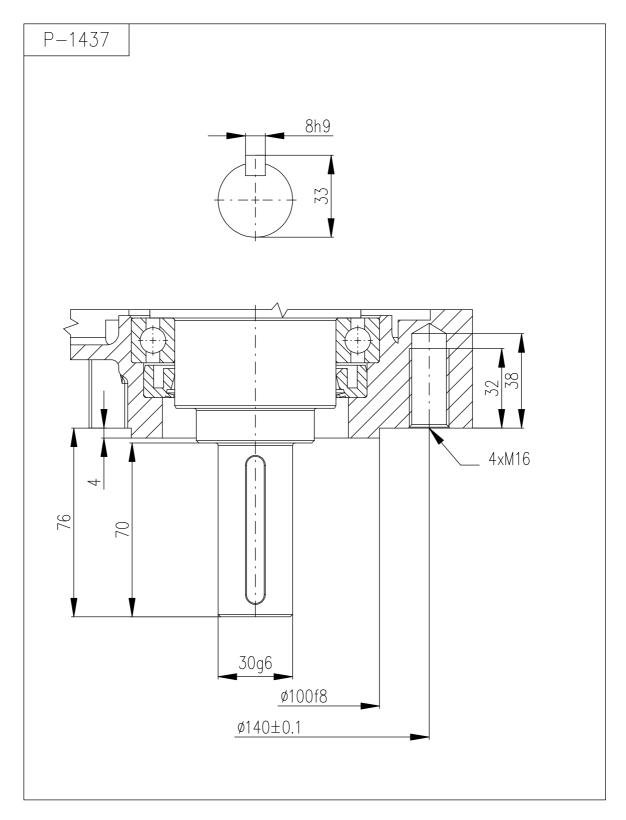
Connection dimensions MO 4 with flange «F14» according to ISO 5210.
