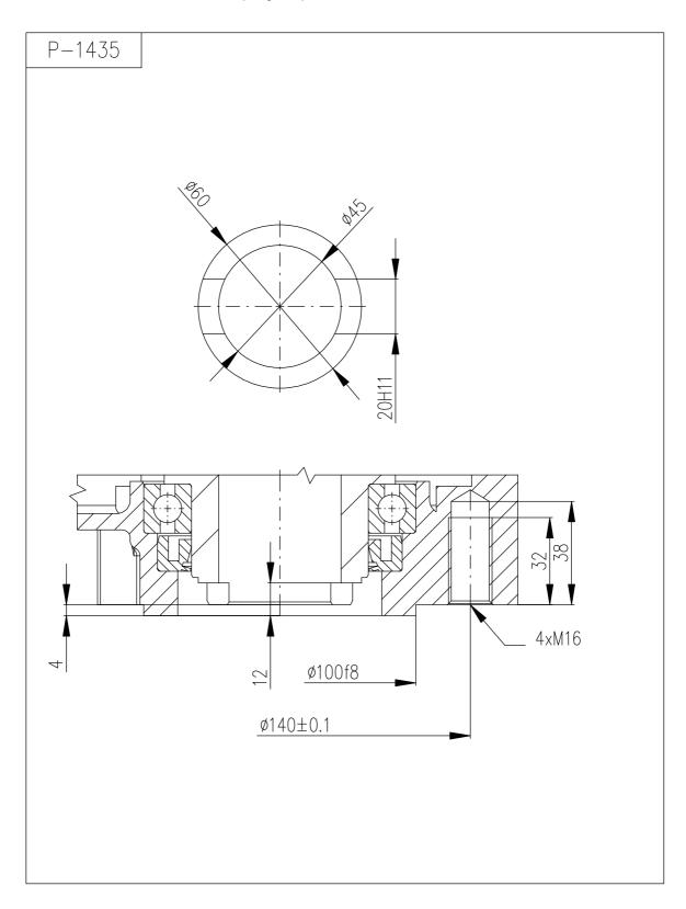
Connection dimensions **MO 4** with flange **«F14»** according to ISO 5210.
